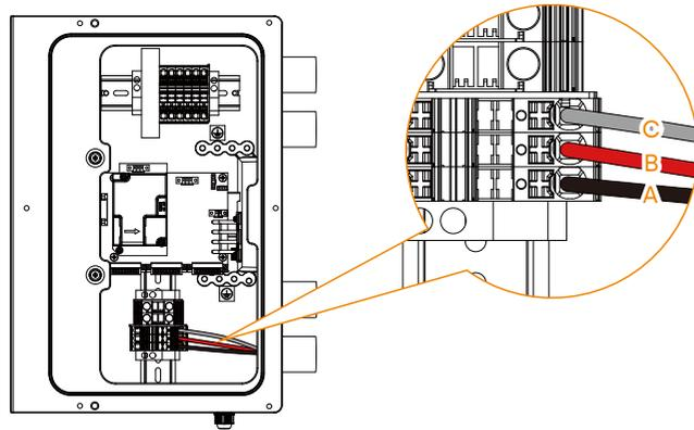
A: L1 cable B: L2 cable C: N cable
