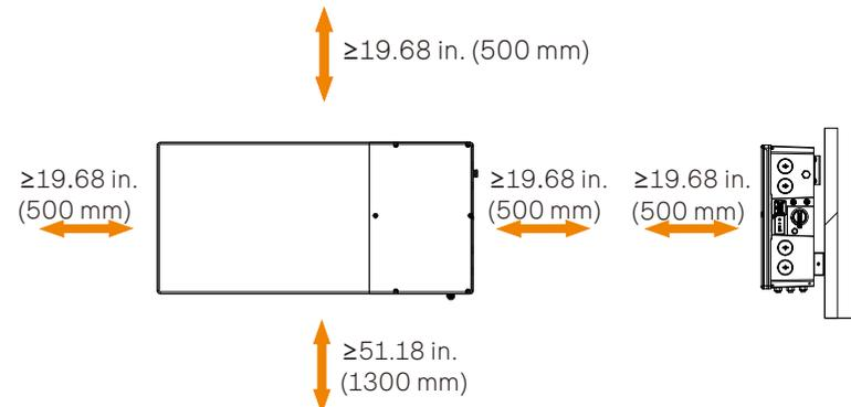
For multi-inverter installation, please reserve the space of 19.68 in. (500 mm) at least between each left and right inverter and at least 19.68 in. (500 mm) space from the ceiling and 51.18 in. (1300 mm) above the ground. If multiple inverters are mounted in areas with high ambient temperatures, increase the clearances between the inverters and ensure an adequate fresh-air supply if possible.
