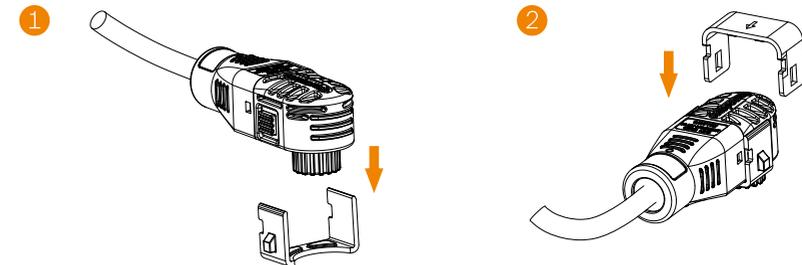
Step 3: Disconnect the series wiring terminal on the battery.
