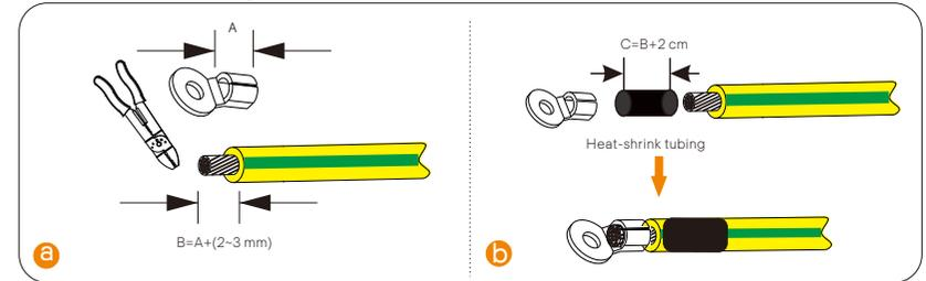
c) Crimp it with crimping tool, pull the heat-shrink tubing over the stripped section of the grounding terminal and use a hot-air blower to shrink it so that it can be firmly contacted with the terminal;
