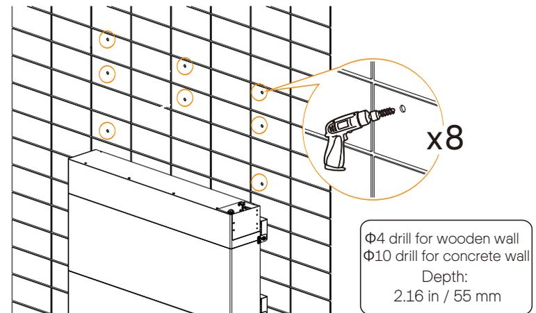
c) Insert the expansion tube(Part I) into the hole and use rubber hammer to knock the expansion tube into the wall. (This step is not required in case of wooden wall.)
