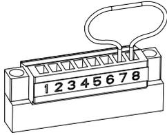
Step 2: Use minimum 24 AWG conductors to connect Pin 7 and Pin 8 (labeled “12V” and “STOP\_NO”) to a suitable emergency stop switch.
