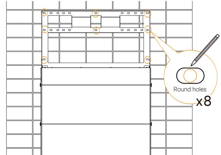
c) Unscrew the two M4 screws to disassemble the bracket. Drill holes with power drill, and make sure the holes are deep enough (2.1 in. / 55.0 mm) to support the inverter.
