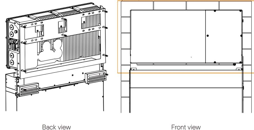
b) Place the cable protective guard(Part N) on the correct position of battery's BMS prior to the wiring connection between inverter and battery and secure it on the inverter's bracket with M5 screws(Part C);
