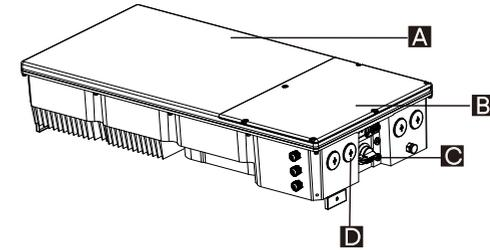
A-Inverter power box: It is the essential part of the inverter. This part is debugged and sealed before ex-factory and there is no user-servable part inside this part. Opening the part is prohibited.
