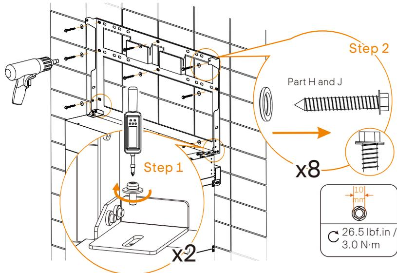
Step 2: Hang and fix the inverter on the bracket
