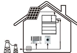
In this work mode, the battery will be charged at the set time and will never discharge when the grid is on. You can also choose whether to charge from the grid or not.
