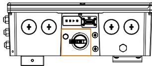
Step 2: Make sure the breaker of battery is in OFF position.
